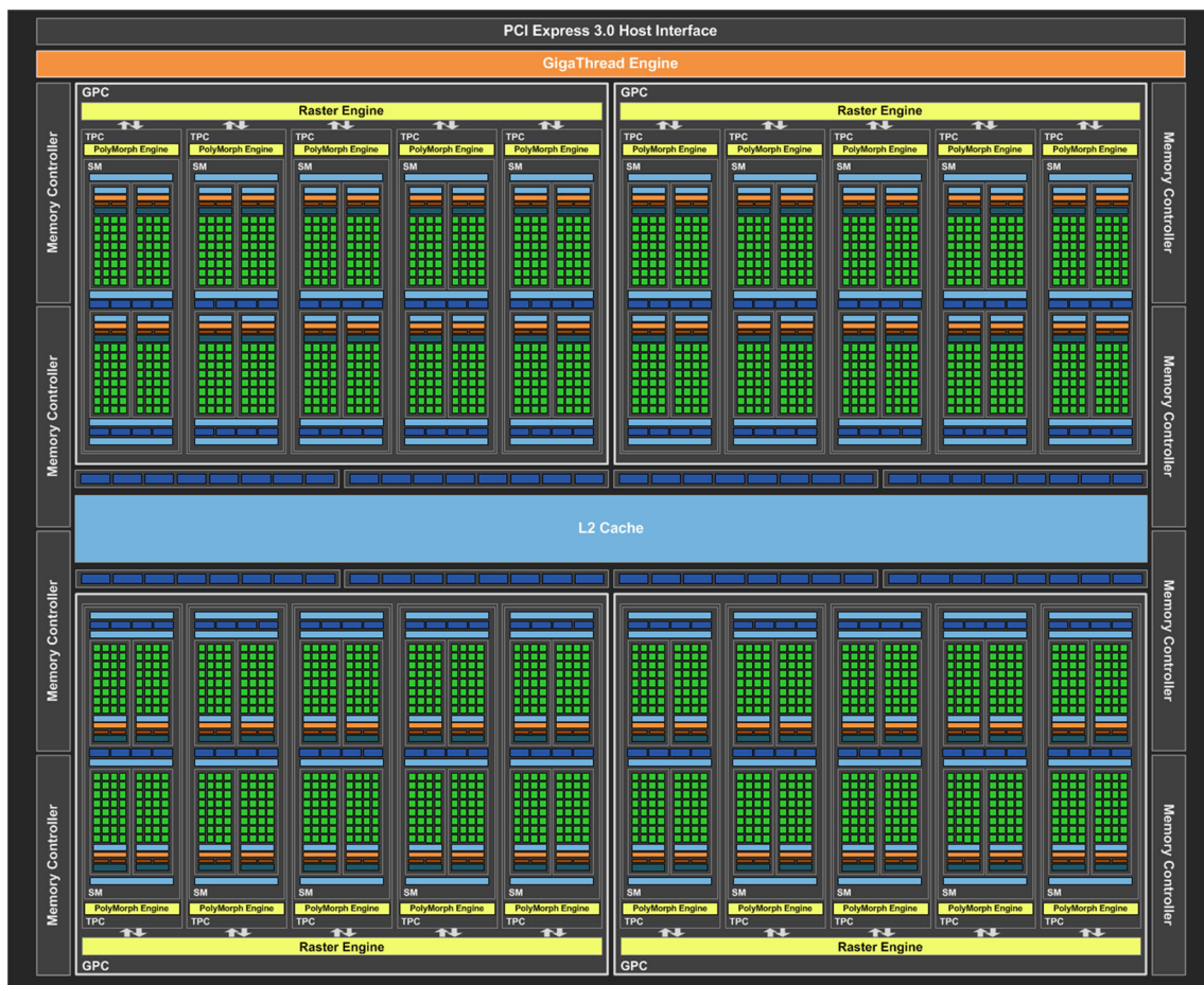
Fig. 1 Block diagram of the GP104 Nvidia GPU core. Green squares are CUDA cores organized into 20 Streaming Multiprocessors (SM). Each SM combines 128 CUDA cores, 256 KB register file, 96 KB of shared memory, 48KB of L1/texture cache and eight texture units (color figure online)
